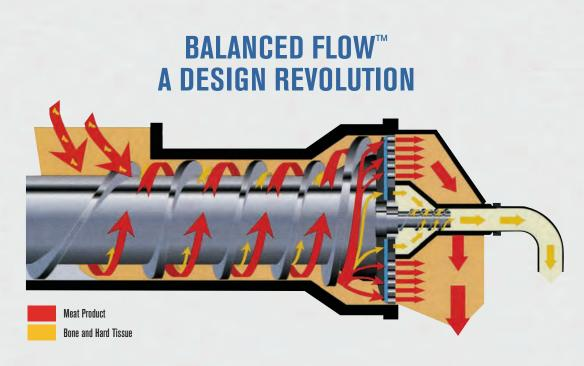
The exclusive Balanced Flow<sup>™</sup> design perfectly balances the volume of product being delivered to the plate relative to open hole area in the plate.
